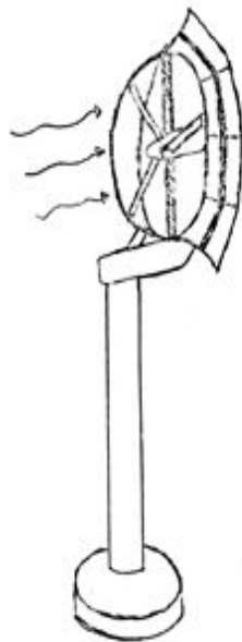
Figure 5: Downwind Turbine with Shroud to increase flow velocity through blades.
